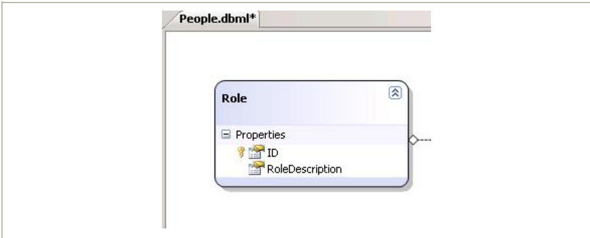
Figure 2-21. The Role table is transformed into the Role entity class after dragging and dropping the table from Server Explorer.
